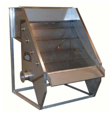
**STATIC SCREEN** is the curve stainless wedge wire hydrostatic screen used for solidliquid separation. The specially designed non-clog hydrostatic screen, with great opening area, offers an economical separation process with more hydraulic capacity, higher efficiency and needs low maintenance. It is used in many different industries and for many different applications.
